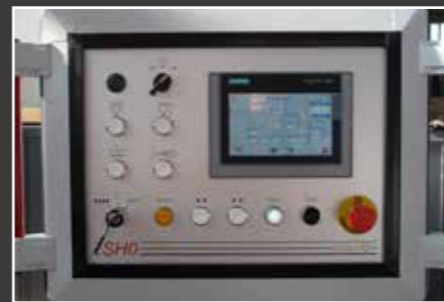
TOUCH-SCREEN CONTROL PANEL
