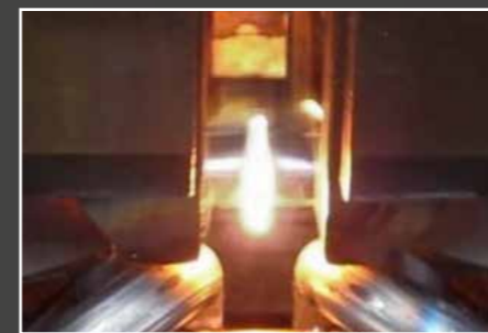
WELDING AND UPSETTING PHASE
