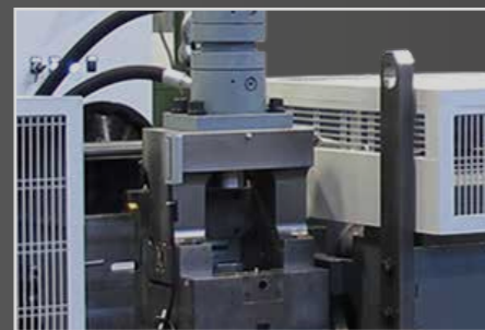
INTEGRATED STAMPING UNIT WITH 4 INDEXING POSITIONS
